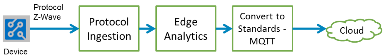
Figure 21 : Z Wave Architecture
