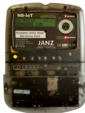
Fig ANNEX2.1: Energy Meter [A2.5]
