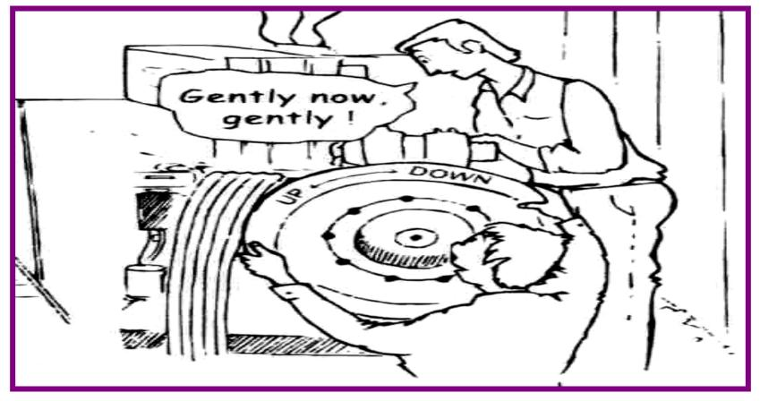
The hand wheel is rotated to drive the elevator car manually. (The rescue person to check which direction is easier to hand wind the lift. If the car is heavier, an assistant can help him.)
