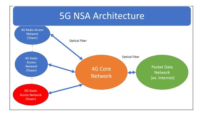
Worldwide operators have launched 5G using NSA architecture of 5G initially based on 3GPP release 15 version of 5G. Now they are migrating their network to 5G Standalone Architecture. This Architecture is also called option 3 deployment of 5G. We will talk about various options later in this article.
